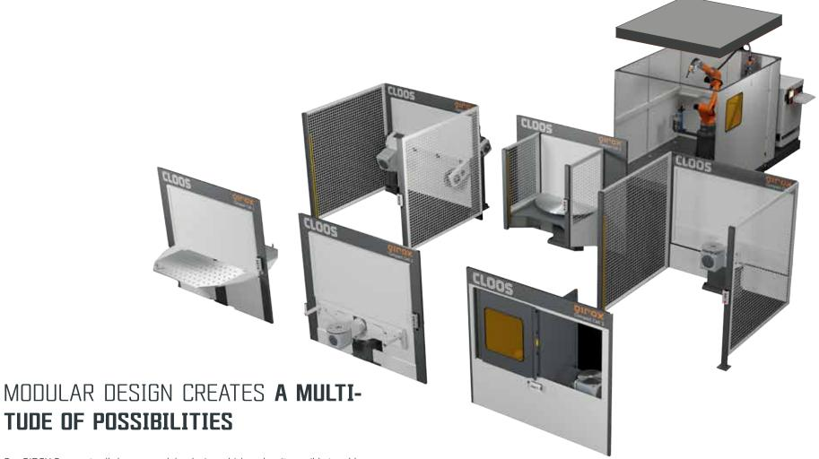
Our QIROX Compact cells have a modular design which makes it possible to add individual enhancements and upgrades – easily, quickly and with minimum expenditure. Thus you can upgrade your QR-CC-1, for example, to a more efficient QR-CC-4 at any time. Benefit from a maximum production flexibility!
